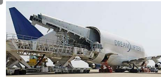
Loading Boeing 787 components to a specialized transport aircraft (Boeing 747 "Dream Lifter")
